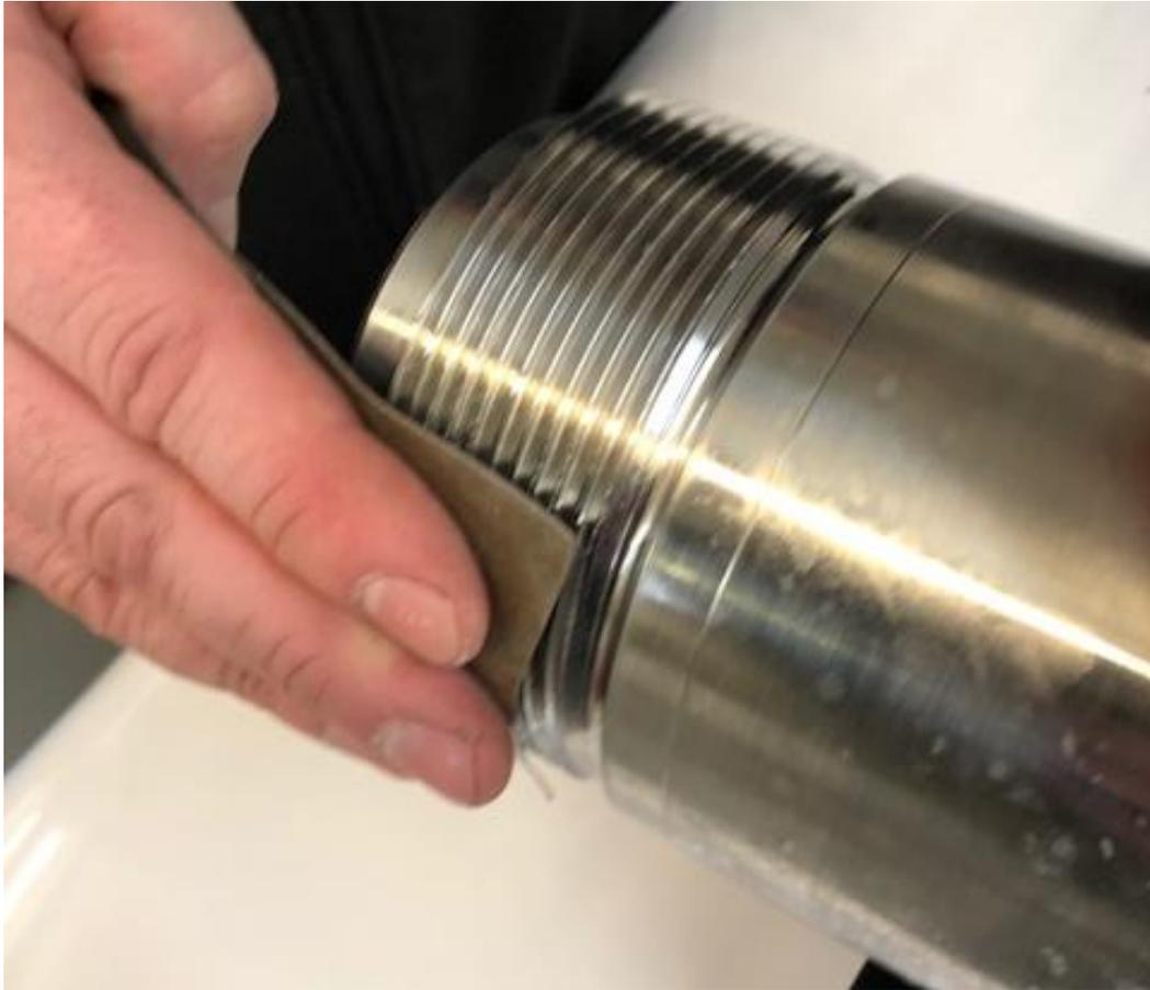
**Hydraulic high pressure cylinder preparation (if not new)**
